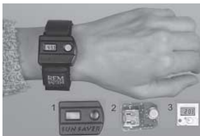
Figure 3. Personal, electronic, UVR dosimeter “SunSaver” worn on the wrist. 1: The housing, 2: The UVR data logger with the sensor and battery, 3: The watch, a separate unit. (Heydenreich and Wulf, 2005).
