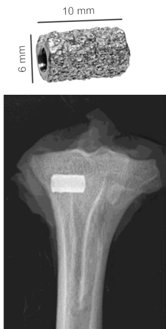
Figure 1. Study I. Press-fit implant model. Press-fit implant device, dimension 10x6 mm. Implant inserted in a 0.1 mm undersized bone bed in the left proximal tibia. X-ray image at time of bone harvest completing 4 weeks treatment of PTH/control.
