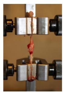
The anastomosis is pulled apart at a constant speed of 10 mm/min.
