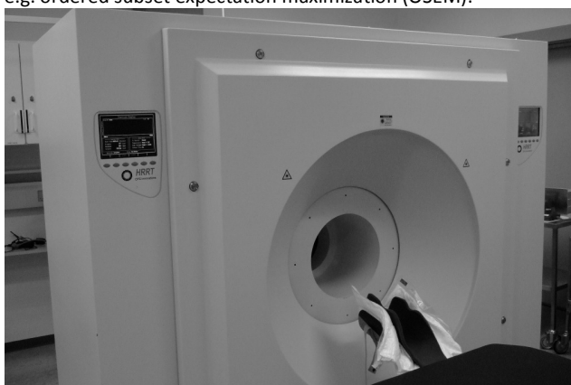
Figure 3 The High Resolution Research Tomograph (HRRT) from Siemens at PET and Cyclotron Unit, Copenhagen University Hospital Rigshospitalet enables PET images with a theoretical resolution of a few millimeters.
