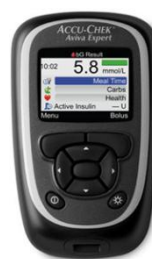
Figure 3 Automated Bolus Calculator. Accu-Chek Aviva Expert is a trademark of Roche. © Roche 2012.
