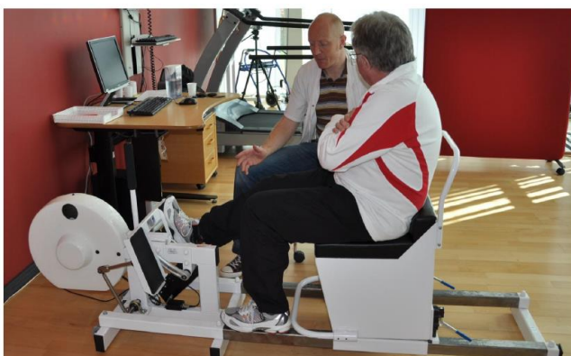
Figure 9. Multi-joint leg extension power evaluated with the Nottingham Power Rig.
