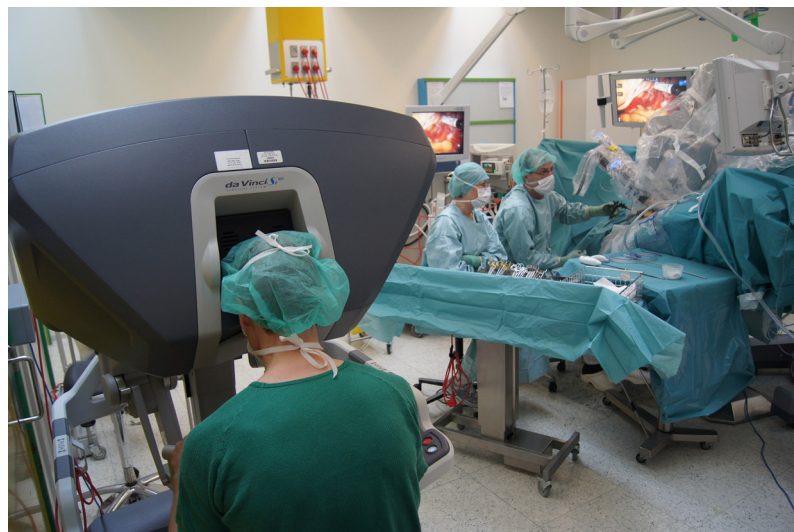
The da Vinci robot with the surgeon console from where all instruments are controlled.
